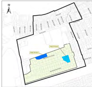
OPTION 1 Construct One Stormwater Management Facility Within the Bay Sands Development Area Using 5 Lots
