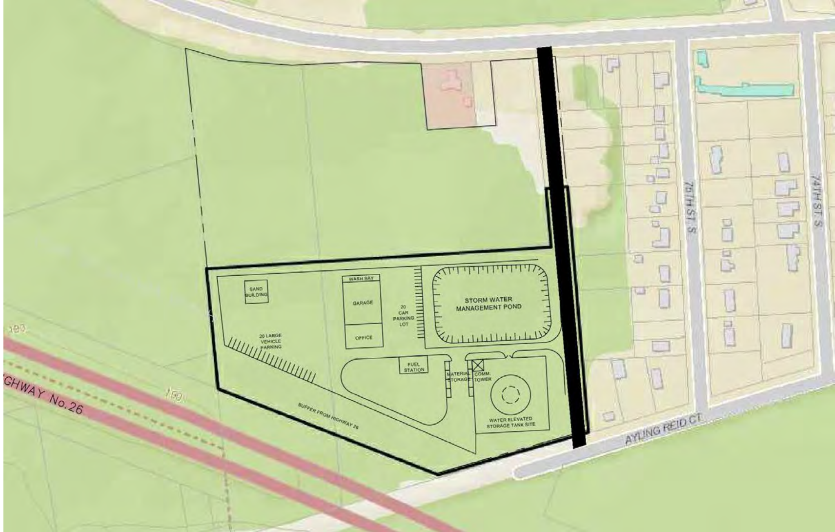
Figure 17 – Alternative 4: SWMP only servicing the maintenance depot and located on the maintenance depot site
