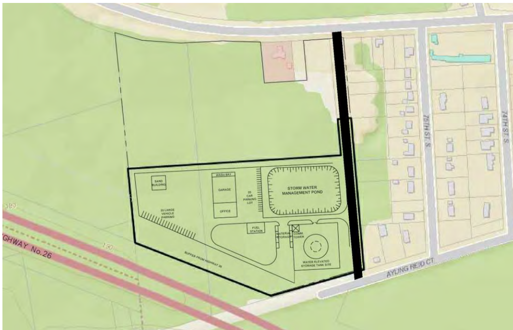
Figure 4 - Alternative 4: SWMP only servicing the maintenance depot and located on the maintenance depot site
